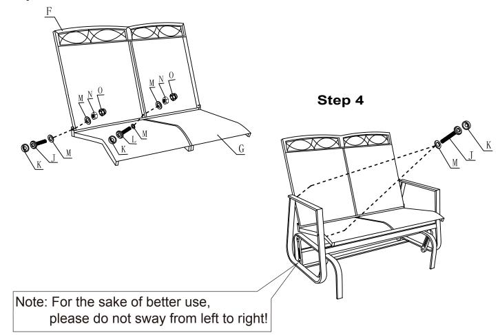
PLEASE ENSURE ALL FIXINGS ARE LEFT LOOSE DURING ASSEMBLY, BUT ARE SECURELY TIGHTENED UPON COMPLETION.
